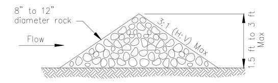
TYPICAL ROCK CHECK DAM SECTION
